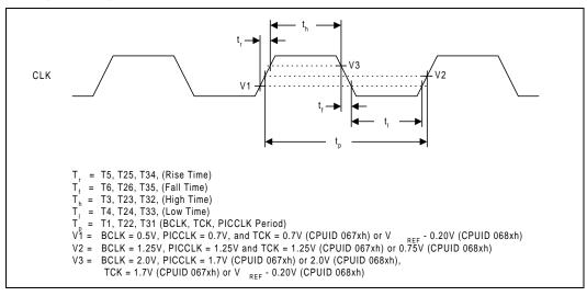
Figure 8. System Bus Valid Delay Timings
