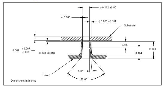
Figure 35. S.E.C.C.2 Packaged Processor Assembly — Side View
