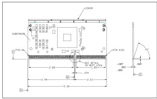
Figure 37. S.E.C.C.2 Packaged Processor Substrate — Edge Finger Contact Dimensions
