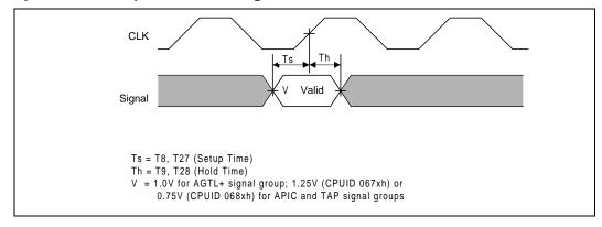
Figure 10. System Bus Reset and Configuration Timings
