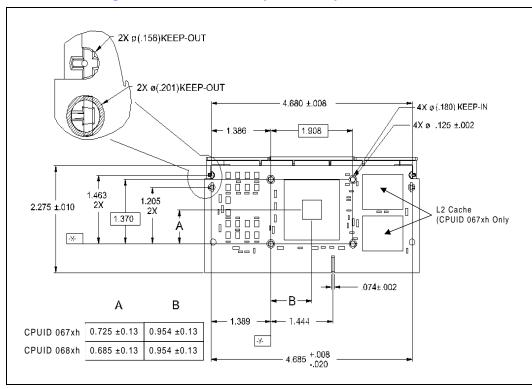
Figure 32. S.E.C.C.2 Packaged Processor Assembly — Primary View
