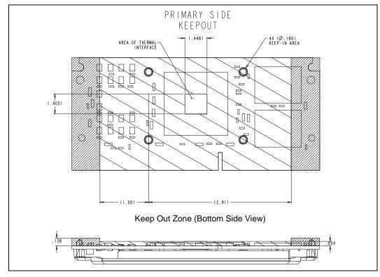
Figure 41. S.E.C.C.2 Packaged Processor Substrate (CPUID 067xh) — Keep-Out Zone
