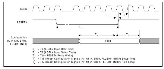
Figure 11. Power-On Reset and Configuration Timings
