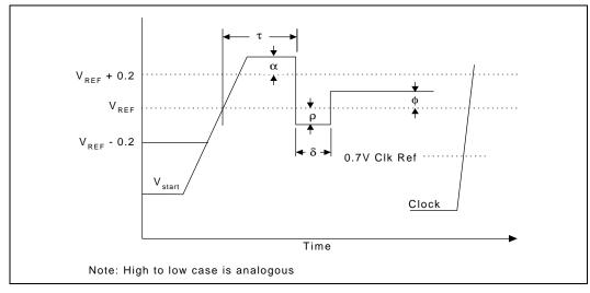
Figure 16. Low to High AGTL+ and Non-AGTL+ Receiver Ringback Tolerance
