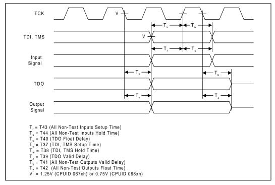
**Figure 13. Test Reset Timings**
