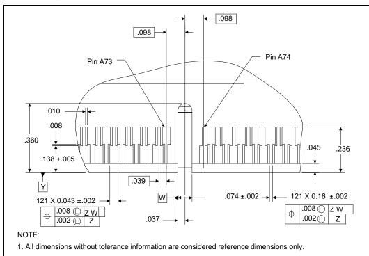
Figure 29. S.E.C.C. Packaged Processor Substrate — Edge Finger Contact Dimensions, Detail A
