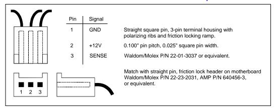
Table 39. Fan Heatsink Power and Signal Specifications
