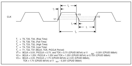
Figure 8. System Bus Valid Delay Timings
