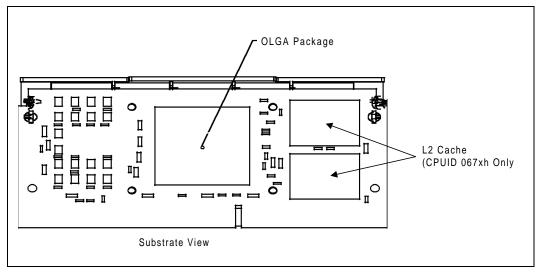
Figure 19. S.E.C.Cartridge 2 — Substrate View
