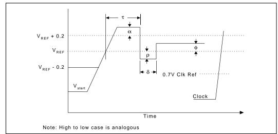
Figure 16. Low to High AGTL+ and Non-AGTL+ Receiver Ringback Tolerance
