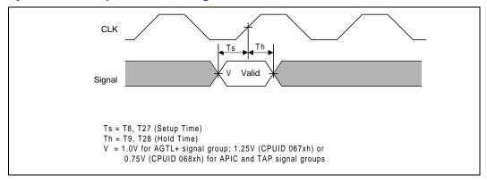
Figure 10. System Bus Reset and Configuration Timings
