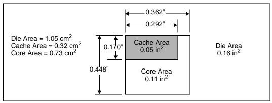
Figure 20. Processor Functional Die Layout (CPUID 068xh)
