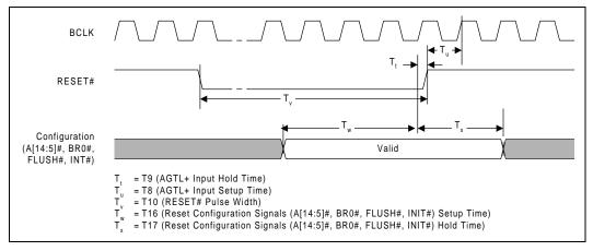
Figure 11. Power-On Reset and Configuration Timings
