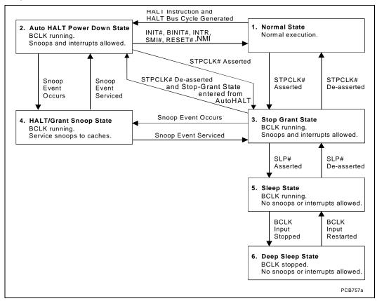
For the processor to fully realize the low current consumption of the Stop-Grant, Sleep and Deep Sleep states, a Model Specific Register (MSR) bit must be set. For the MSR at 02AH (Hex), bit 26 must be set to a '1' (this is the power on default setting) for the processor to stop all internal clocks during these modes. For more information, see the *Intel Architecture Software Developer's Manual, Volume 3: System Programming Guide*.
