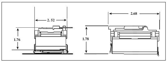
Figure 24. Side View of Space Requirements for the Boxed Processor
