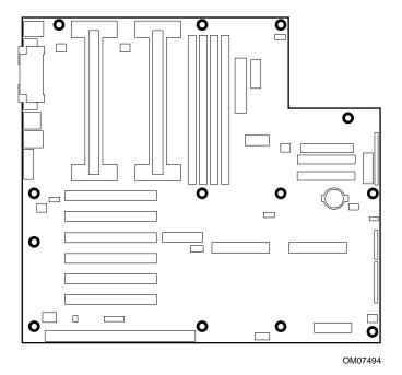
Figure 3. Server Board Screw Hole Locations
