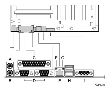
Figure 1. Back Panel Connectors
