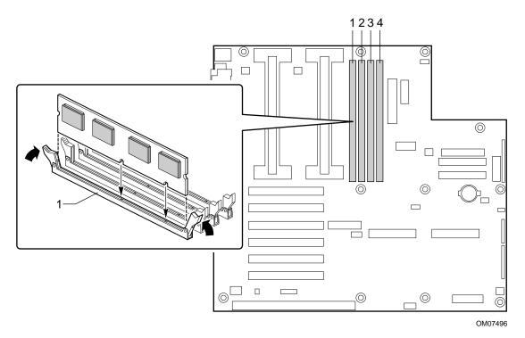
Figure 4. Installing DIMMs
