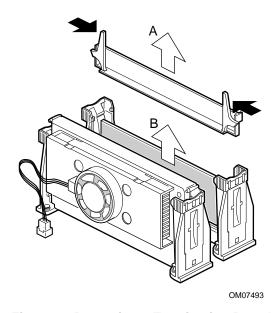
Figure 6. Removing a Termination Board
