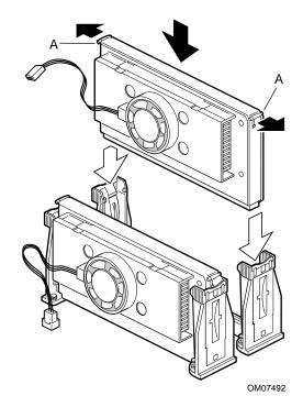
Figure 5. Installing a Processor
