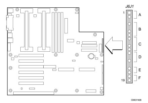
Figure 16. ATX Style Front Panel Connector
