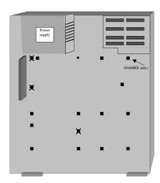
Intel will be making a modification to the "Integrators Guide" for both the Astor 2 and Columbus III to better reflect proper stand-off locations.
