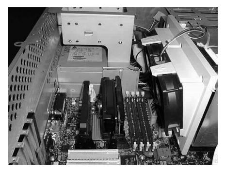
• With your right thumb, push out the top of the white GRM toward the edge of the board. The GRM is very rigid, so only a small amount of tilt is possible.
