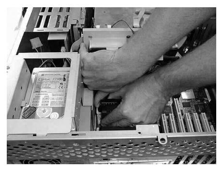
• You should be able to rotate the processor out of the processor slot. Once free of the white GRM, the processor may be removed completely.
