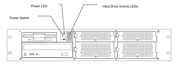
Figure 5. Front Panel and Functions
