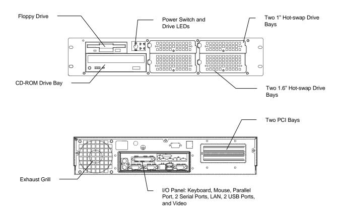
Figure 2. Front and Rear Chassis Views
