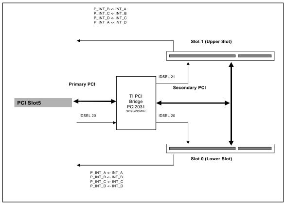
Figure 8. Active PCI Riser Block Diagram
