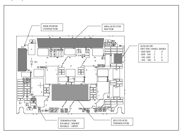
Figure 6. Functional Diagram of the Hot-Swap SCSI Backplane
