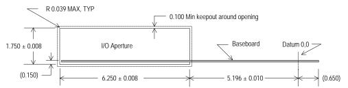
Figure 1. ATX 2.03 I/O Aperture
