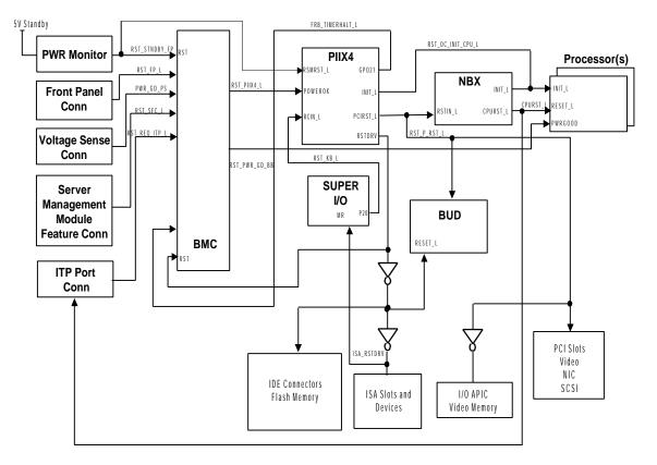
Figure 3-5. Reset Flow Diagram
