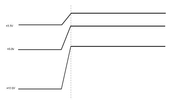
Figure 6-1. DC Voltage Sequencing
