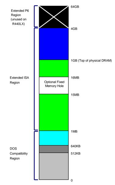
Figure 15. Pentium II processor memory address space
