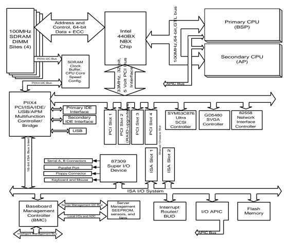
Figure 1 N440BX Server Functional Block Architecture
