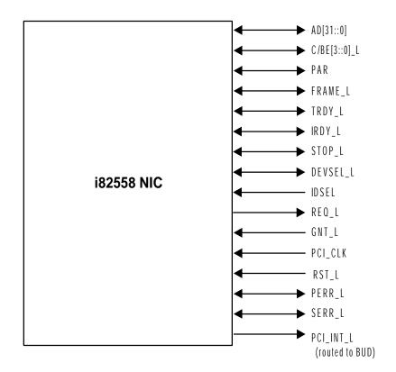
Figure 1-4. Embedded NIC PCI Signals
