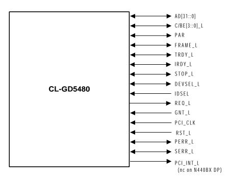
Figure 3-3. Video Controller PCI Signals
