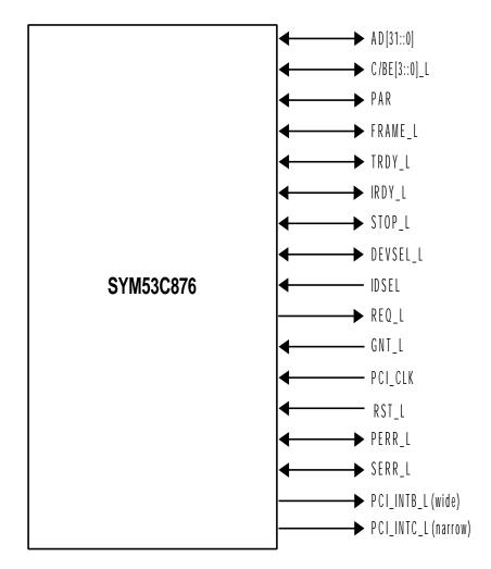
Figure 3-2. Embedded SCSI PCI Signals
