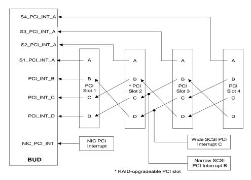
Figure 3-8. PCI Slot Interrupt Swizzle
