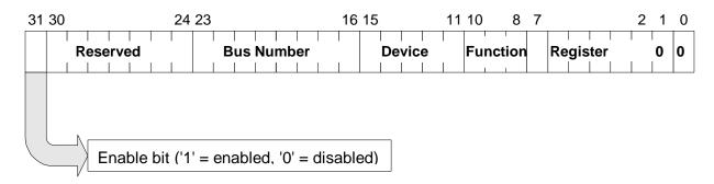
Figure 18 CONFIG\_ADDRESS Register
