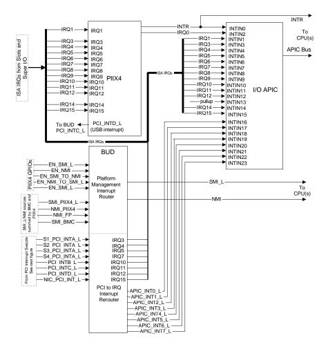
Figure 3-7. Interrupt Structure
