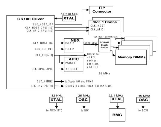
Figure 3-6. Clock Generation and Distribution
