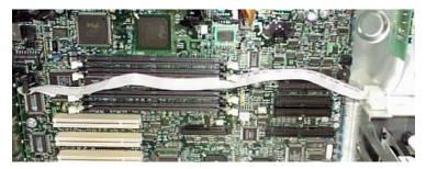
Make sure to stretch the cable that attaches to the drive bay parallel with the DIMM sockets before swinging the SCA hard drive cage into place. Often this cable falls down and can be pinched and damaged when installing the drive bay.
