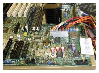
Connect the Astor II chassis power connector to the ATX power connector on the N440BX board. It will look like the picture to the left. Note that there are 4 pins that hang over the edge of the ATX connector on the N440BX baseboard. Also note the black ATX designation on the Astor II power connector.
