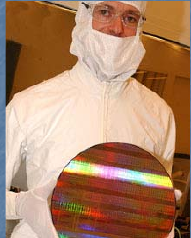
An Intel engineer holding a 300mm wafer with 45nm shuttle test chips.
