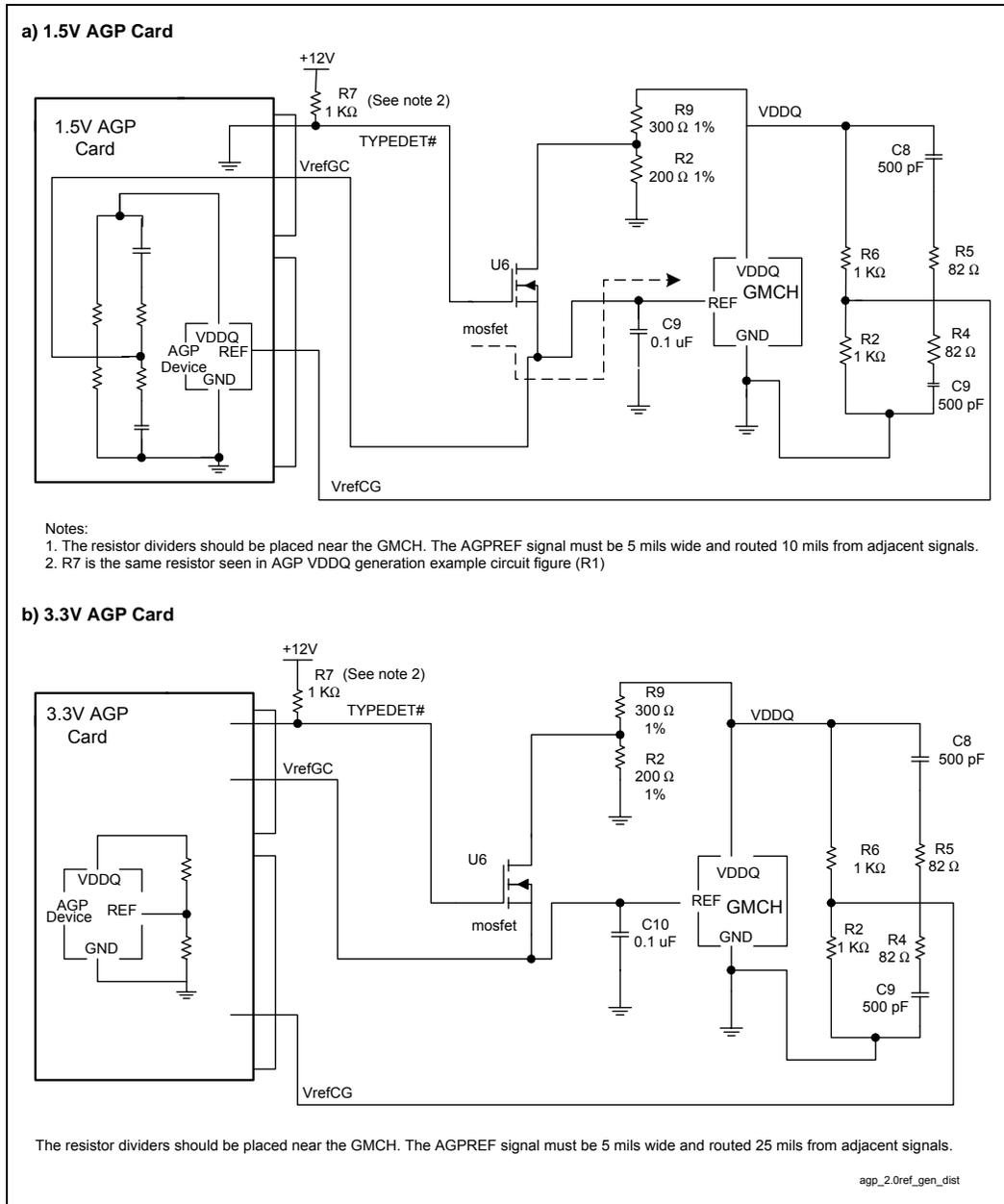
The flexible VREF divider shown in Figure 50 uses a FET switch to switch between the locally generated VREF (for 3.3 V add-in cards) and the source-generated VREF (for 1.5 V add-in cards).
