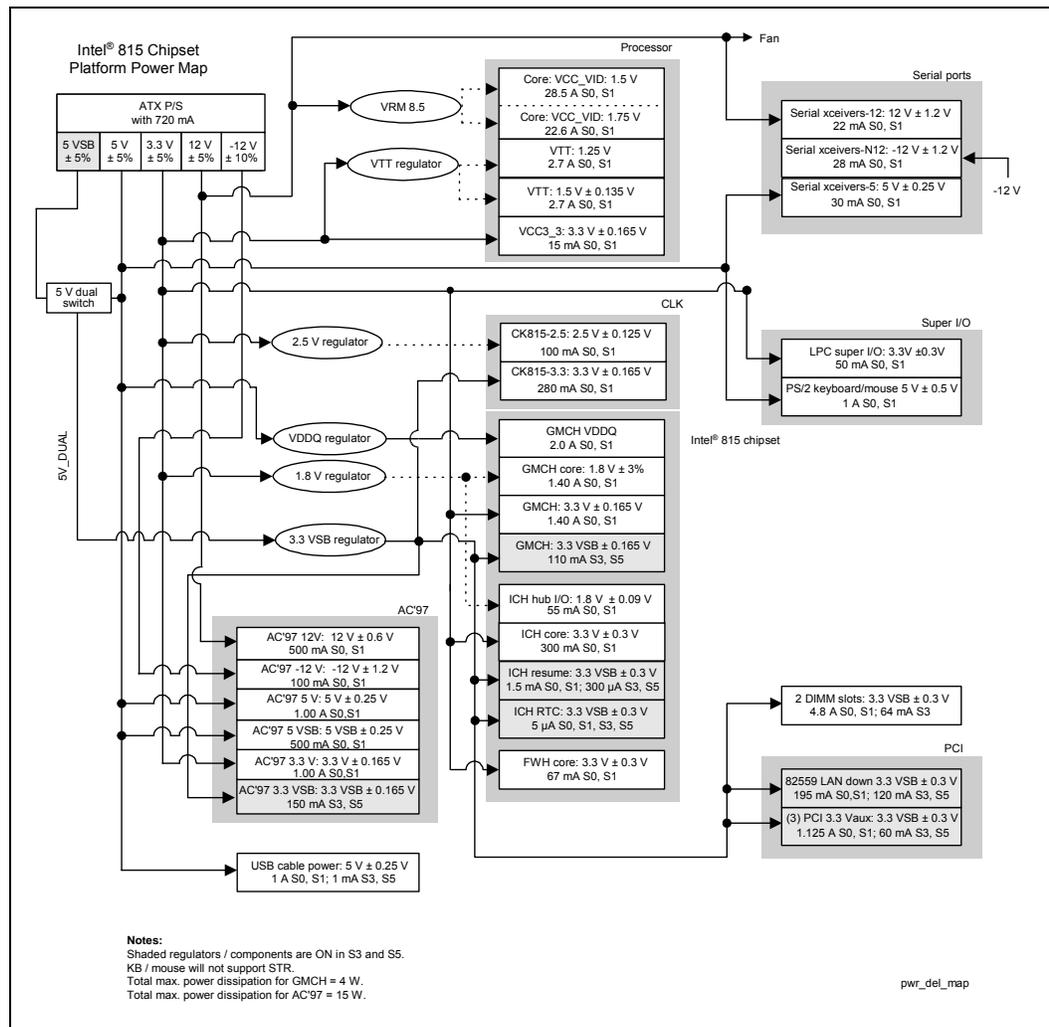
In addition to the power planes provided by the ATX power supply, an **instantly available** 815P chipset platform (using *Suspend-to-RAM*) requires six power planes to be generated on the board. The requirements for each power plane are documented in this section. In addition to on-board voltage regulators, the CRB will have a *5V Dual Switch*.
