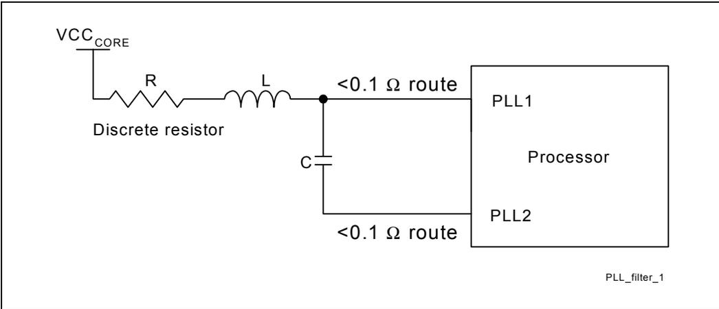
Figure 29. Example PLL Filter Using a Buried Resistor
