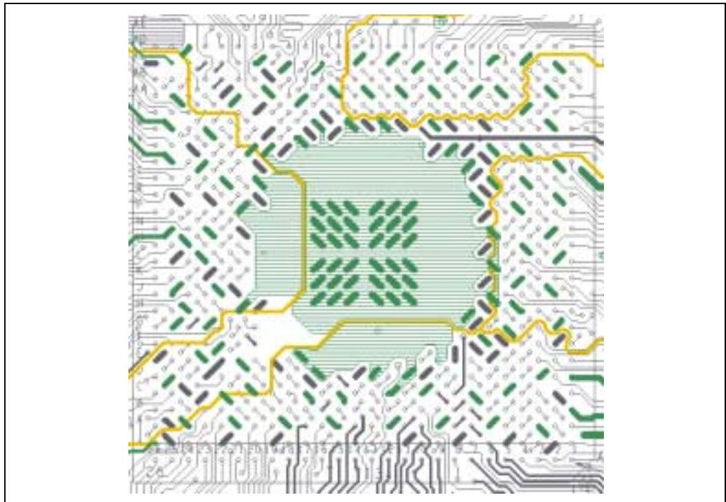
Yellow lines in Figure 42 show layer-two plane splits. (Printed versions of this document will show the layer-two plane splits in the left-side, bottom, right-side, and upper-right-side quadrants)
