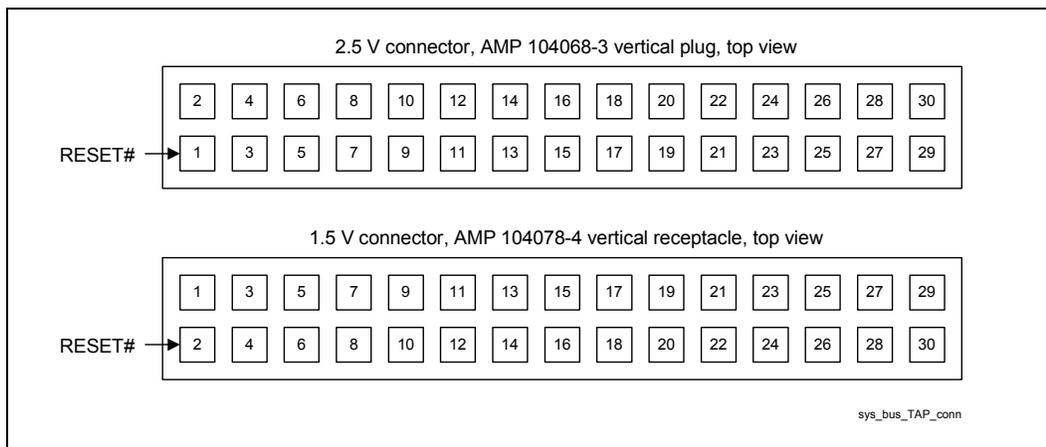
**Caution:** Pentium III processor (CPUID=068xh) and Celeron processor (CPUID=068xh) require an in-target probe (ITP) compatible with 1.5 V signal levels on the TAP. Previous ITPs were designed to work with higher voltages and may damage the processor if connected to any of these specified processors.
