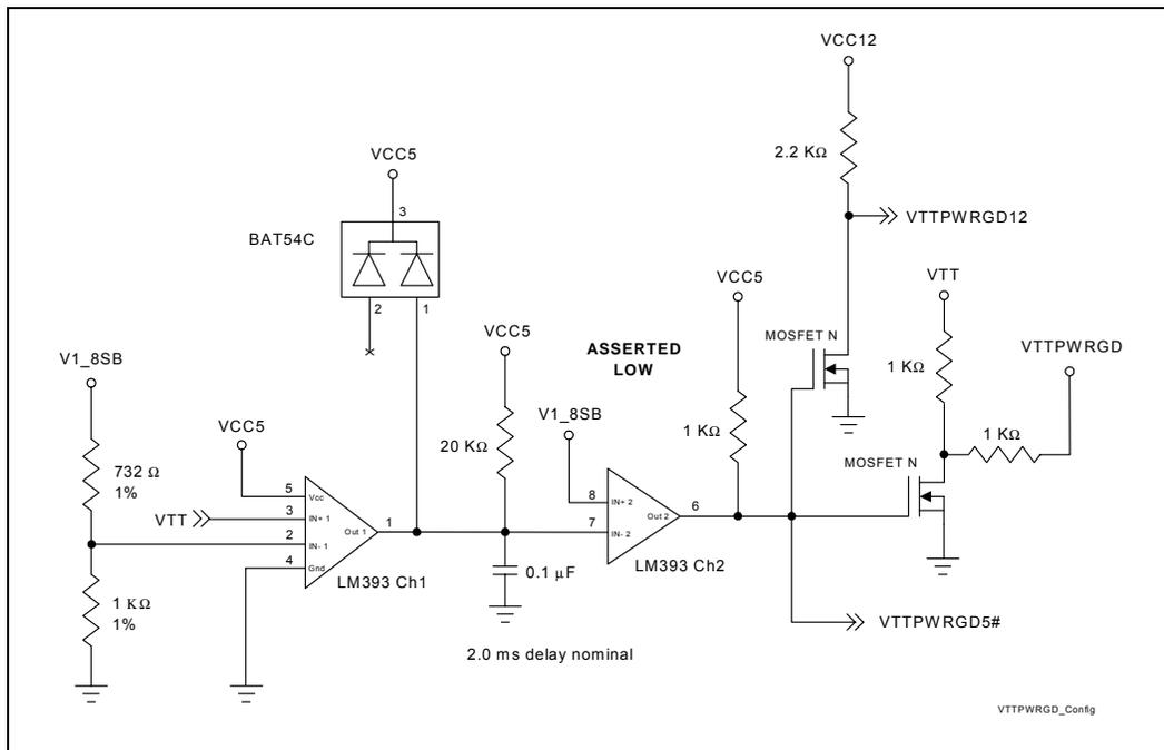
**NOTE:** The diode is included so that repeated pressing of the reset or power button does not cause the capacitor to build up enough charge to circumvent the 20 ms delay.
