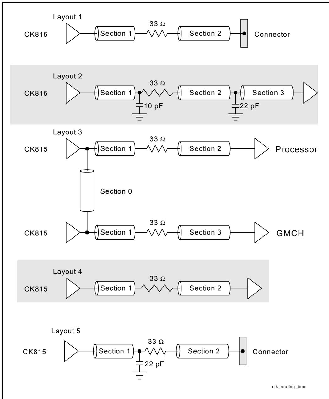
Table 31. Simulated Clock Routing Solution Space
