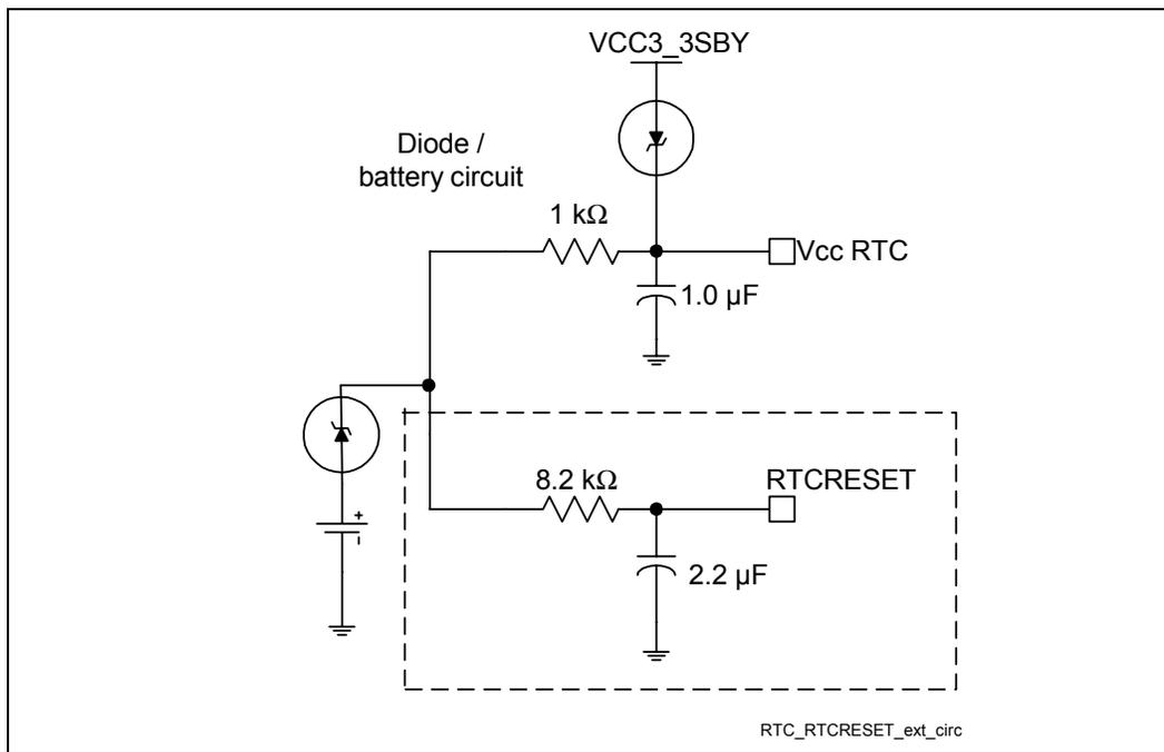
This RTCRESET circuit is combined with the diode circuit (Figure 65), which allows the RTC well to be powered by the battery when the system power is not available. Figure 65 shows an example of this circuitry, which is used in conjunction with the external diode circuit.
