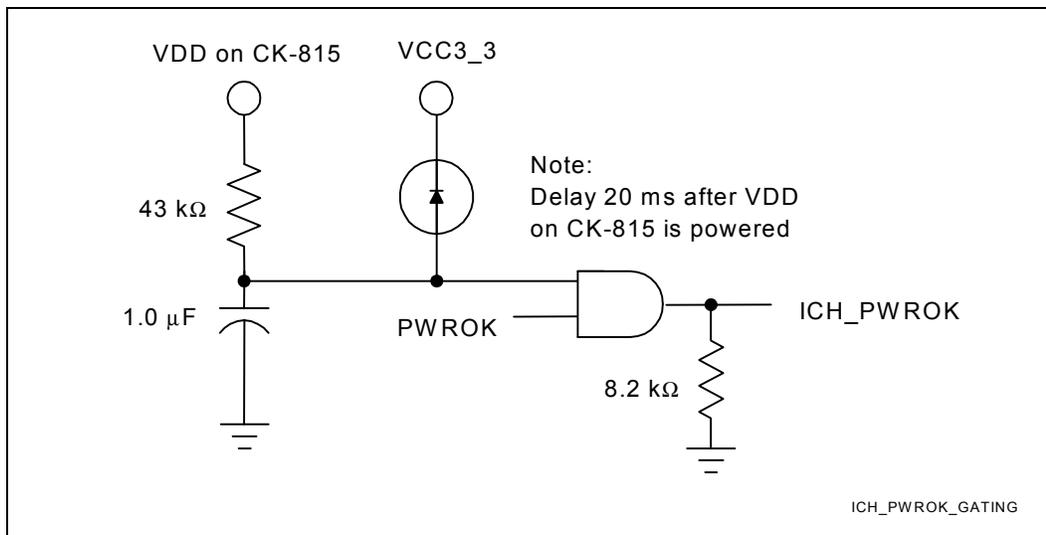
**NOTE:** The diode is included so that repeated pressing of the reset or power button does not cause the capacitor to build up enough charge to circumvent the 20 ms delay.
