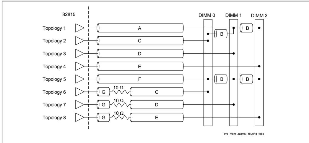
In addition to meeting the spacing requirements outlined in Table 20, system memory signal trace edges must be at least 30 mils from any other non-system memory signal trace edge.
