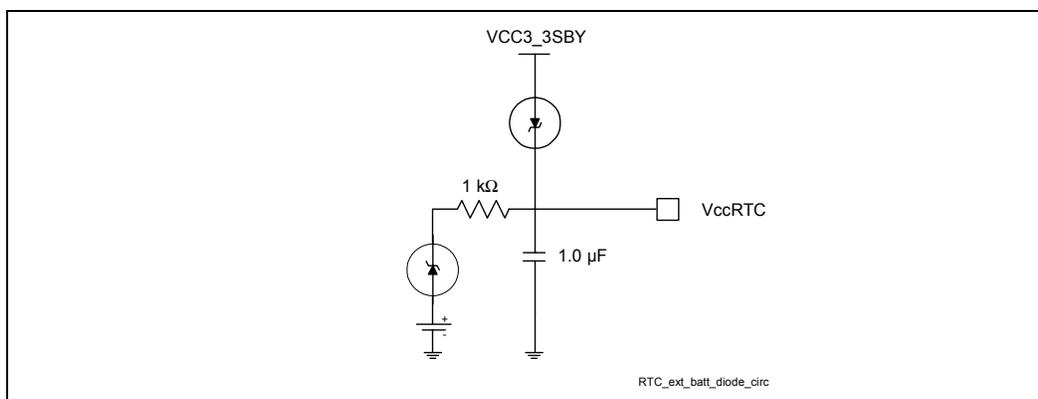
A standby power supply should be used to provide continuous power to the RTC when available, which will significantly increase the RTC battery life and thereby the RTC accuracy.
