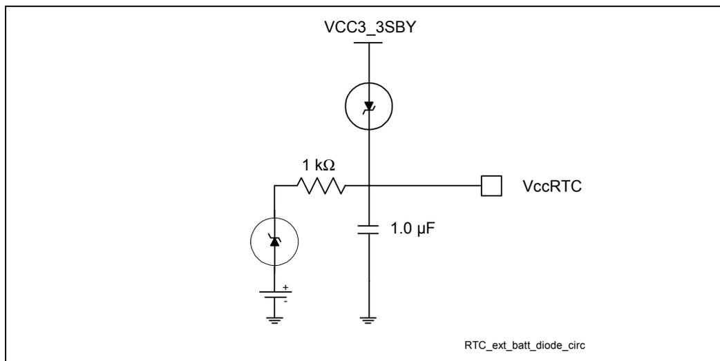
A standby power supply should be used in a desktop system, to provide continuous power to the RTC when available, which will significantly increase the RTC battery life and, thereby, the RTC accuracy.
