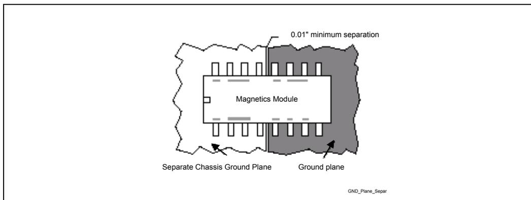
Good grounding requires minimizing inductance levels in the interconnections. Keeping ground returns short, signal loop areas small, and power inputs bypassed to signal return significantly reduces EMI radiation.
