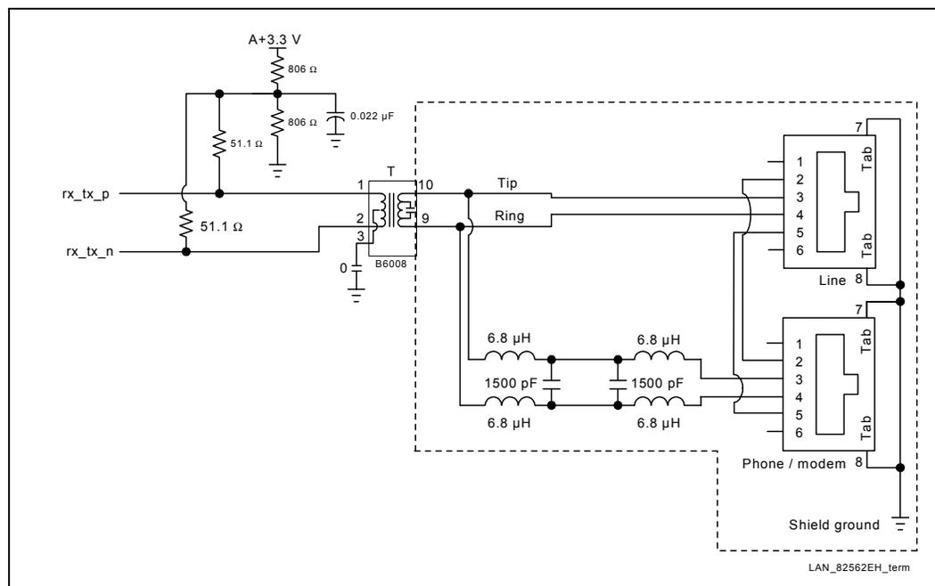
The filter and magnetics component T1 integrates the required filter network, high-voltage impulse protection, and transformer to support the HomePNA LAN interface.
