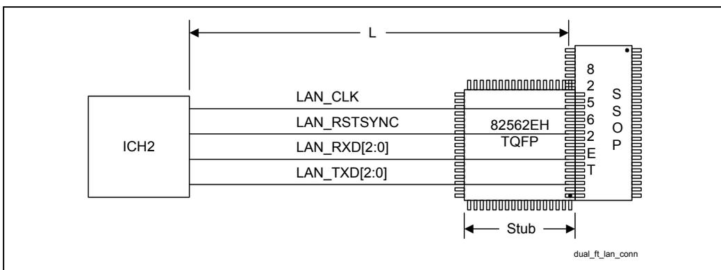
**Figure 96. Dual-Footprint Analog Interface**
