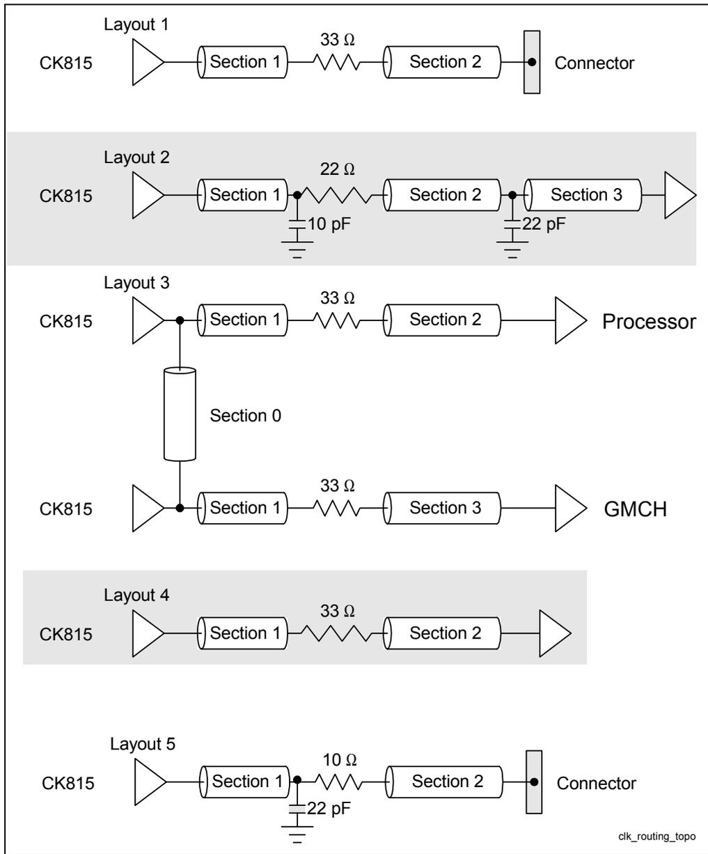
Table 42. Simulated Clock Routing Solution Space
