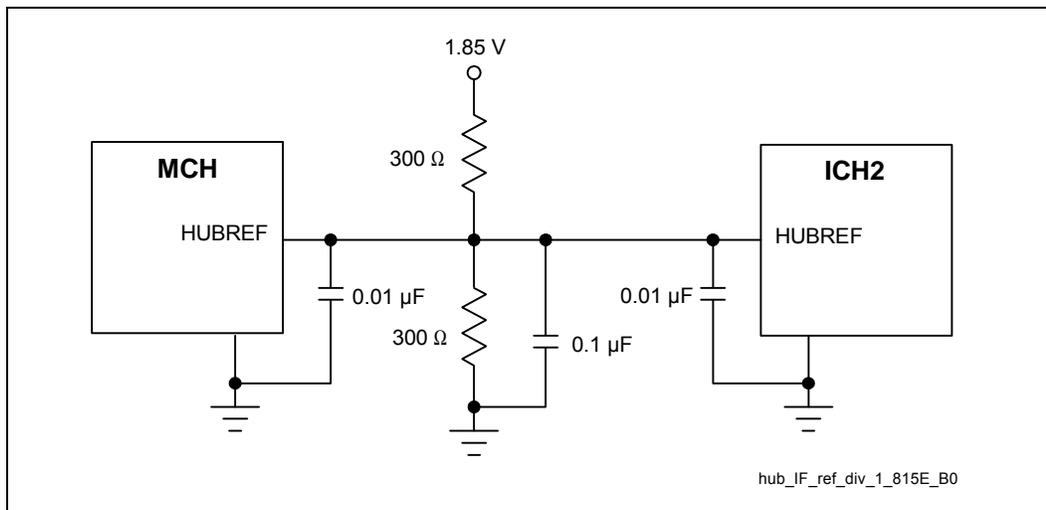
**Figure 58. Locally Generated Hub Interface Reference Dividers**
