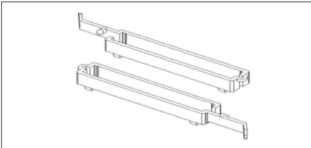
**Figure 50. AGP Left-Handed Retention Mechanism Keep-Out Information**
