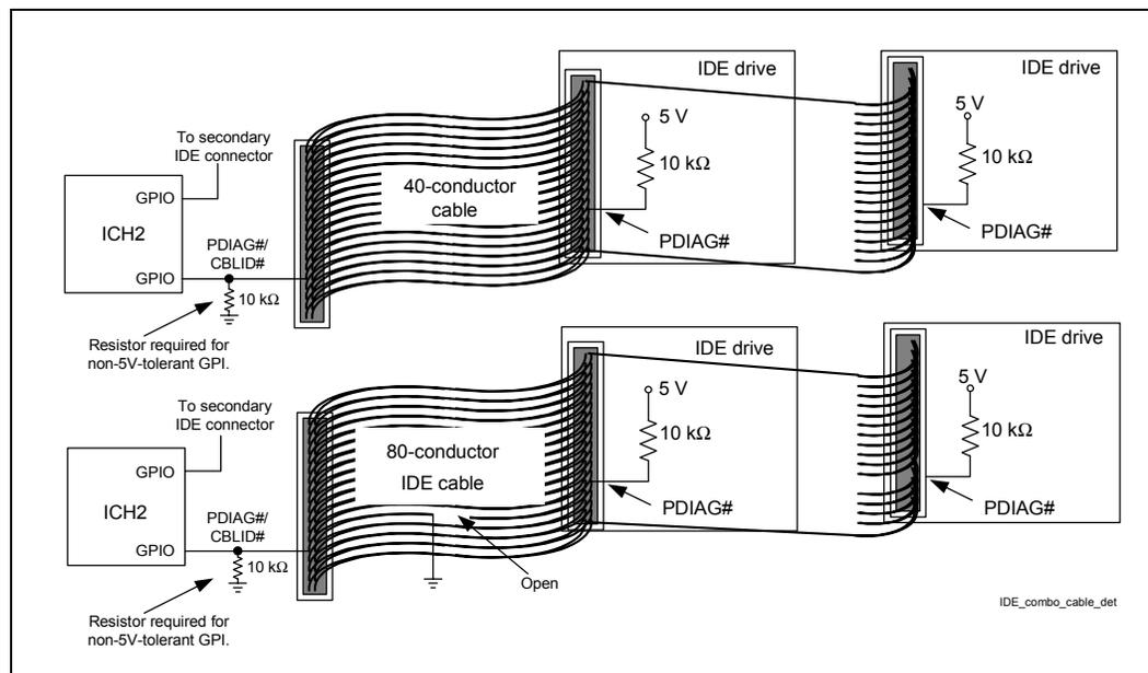
This mechanism allows BIOS, after diagnostics, to sample PDIAG#/CBLID#. If the signal is High, then there is 40-conductor cable in the system and ATA modes 3, 4 and 5 must not be enabled.
