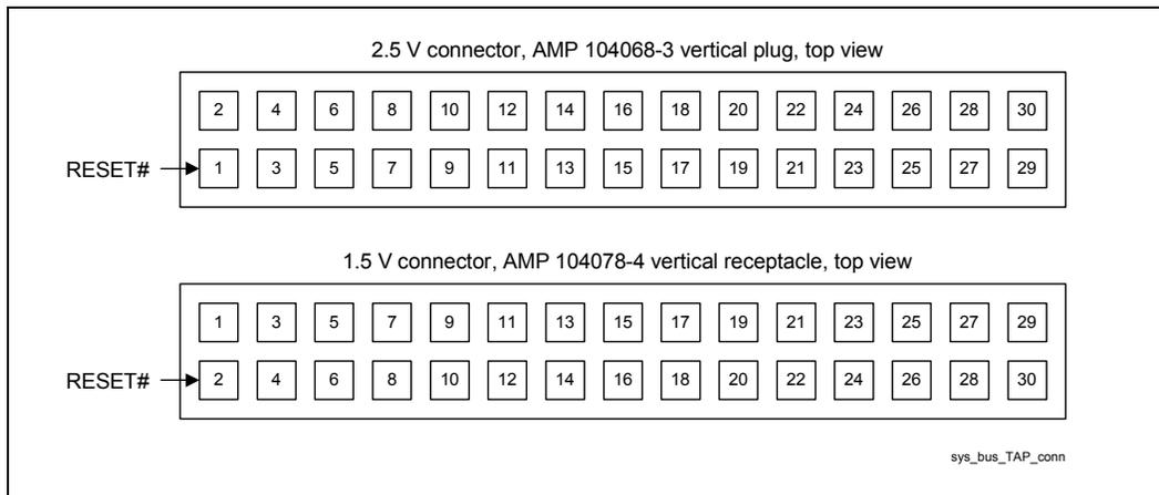
**Caution:** The Pentium III processor (CUID=068xh) and Celeron processor (CUID=068xh) require an in-target probe (ITP) compatible with 1.5 V signal levels on the TAP. Previous ITPs were designed to work with higher voltages and may damage the processor if connected to any of these specified processors.
