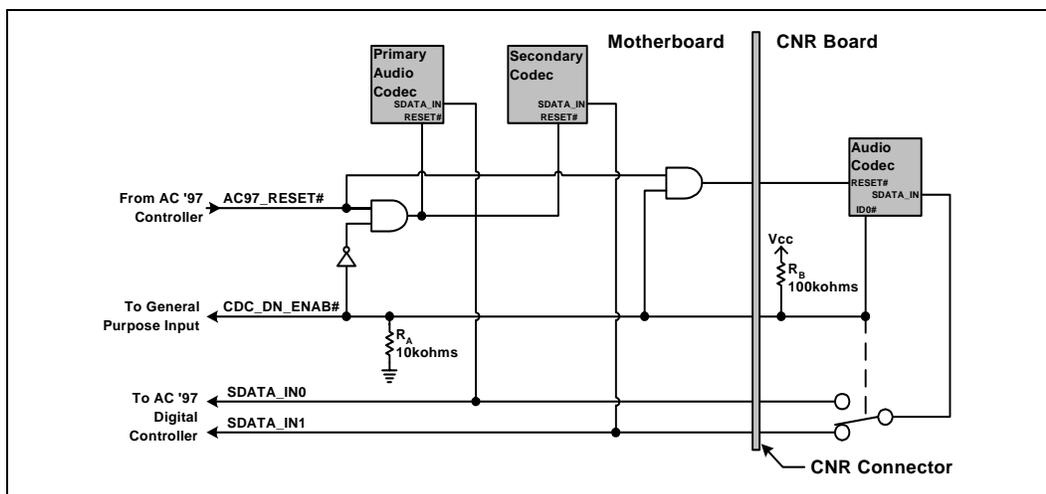
Figure 70 shows the case of two-codex down and a dual-codex CNR. In this case, both codex on the motherboard are disabled (while both on CNR are active) by  $R_A$  being 10 k $\Omega$  and  $R_B$  being 1 k $\Omega$ .
