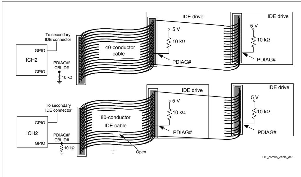
Figure 111. Device Side Only Cable Detection
