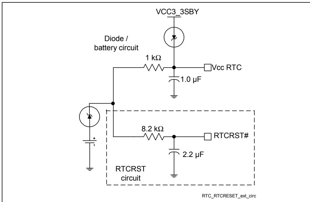
This RTCRST# circuit is combined with the diode circuit (see Figure 81), which allows the RTC well to be powered by the battery when system power is unavailable. Figure 81 shows an example of this circuitry when used in conjunction with the external diode circuit.
