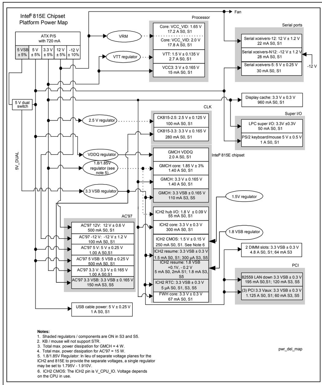
In addition to the power planes provided by the ATX power supply, an *instantly available* 815EP universal platform (using *Suspend-to-RAM*) requires six power planes to be generated on the board. The requirements for each power plane are documented in this section. In addition to on-board voltage regulators, the CRB will have a *5V Dual Switch*.
