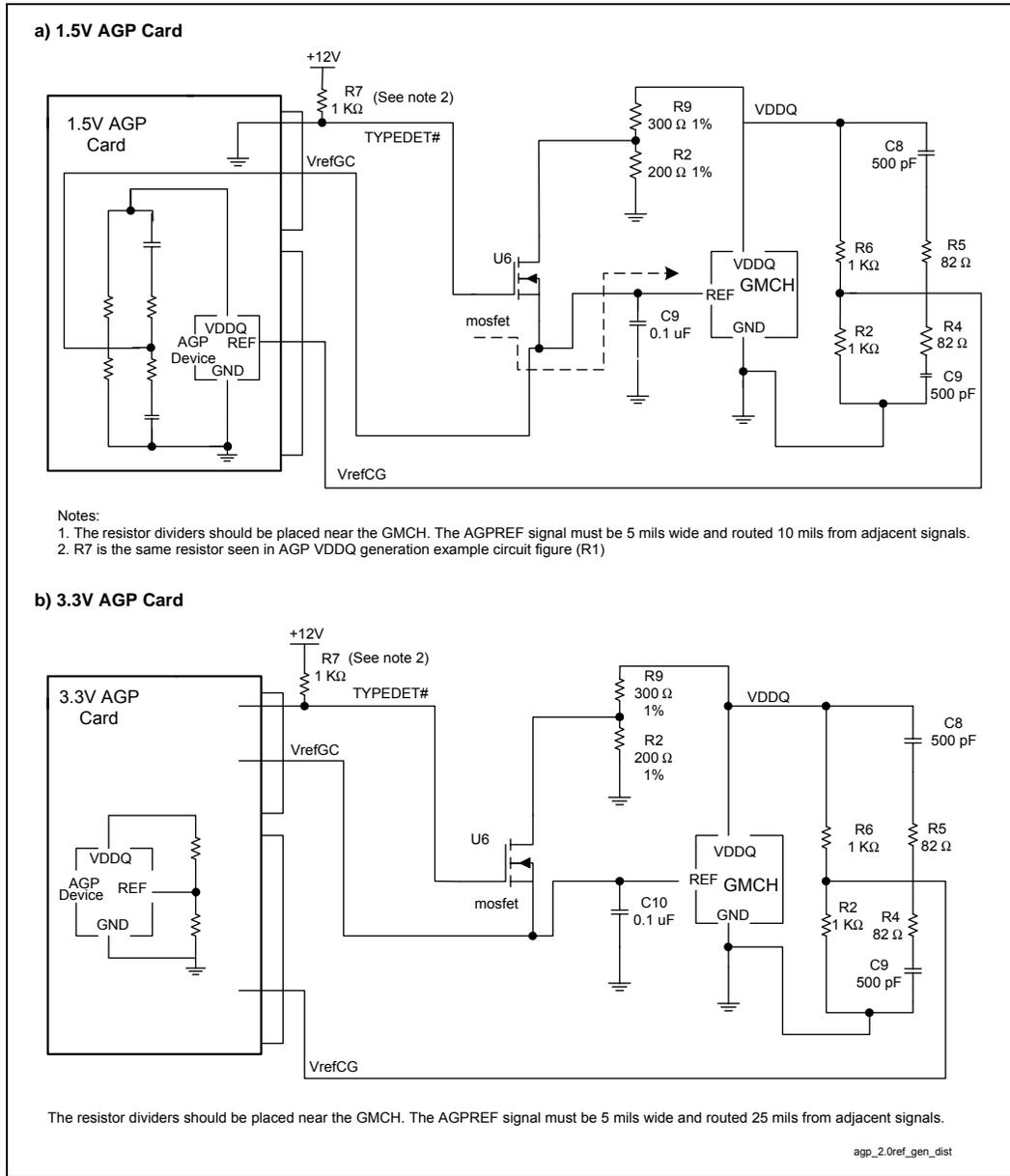
The flexible VREF divider shown in Figure 55 uses a FET switch to switch between the locally generated VREF (for 3.3 V add-in cards) and the source-generated VREF (for 1.5 V add-in cards).
