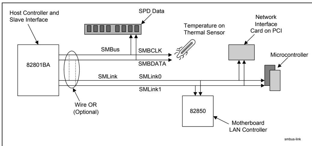
**Note:** Intel does not support external access to the ICH2’s integrated LAN controller via the SMLink interface. Also, Intel does not support access to the ICH2’s SMBus slave interface by the ICH2’s SMBus host controller. Table 33 describes the pull-up requirements for different implementations of the SMBus and SMLink signals.
