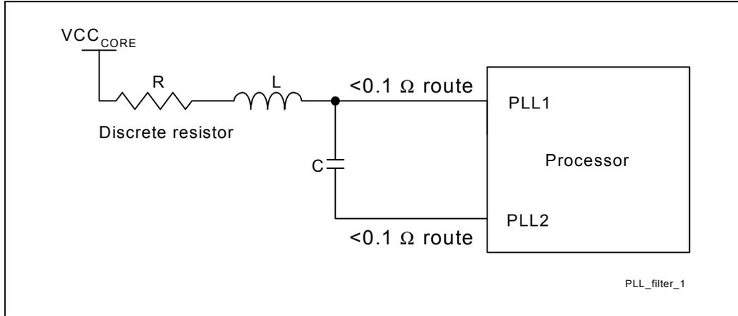
**Figure 34. Example PLL Filter Using a Buried Resistor**
