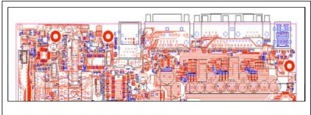
**Figure 6. Top Signal Layer after the Ground Fill Near the I/O Layer**
