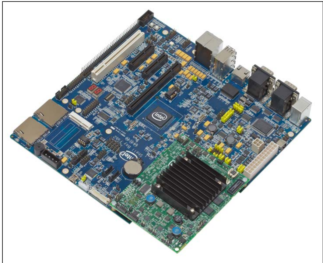
Figure 1. Intel® Atom™ Processor E660 with Intel® Platform Controller Hub EG20T Development Kit
