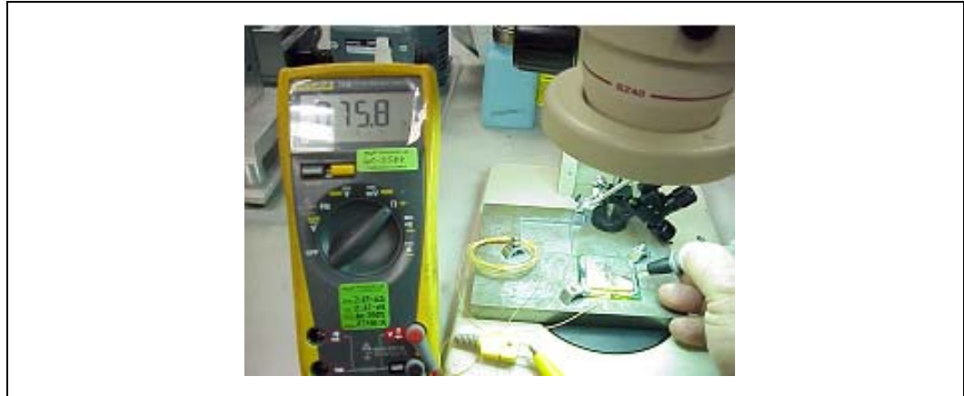
Figure 30. Applying the Adhesive on the Thermocouple Bead
