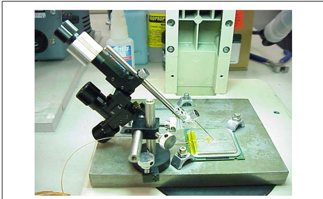
Figure 28. Using 3D Micromanipulator to Secure Bead Location
