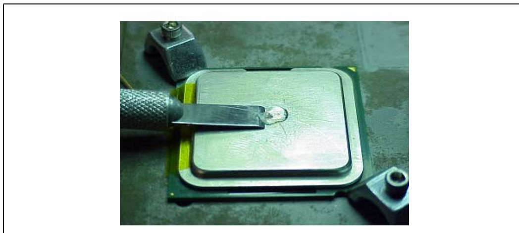
Figure 32. Removing Excess Adhesive from IHS
