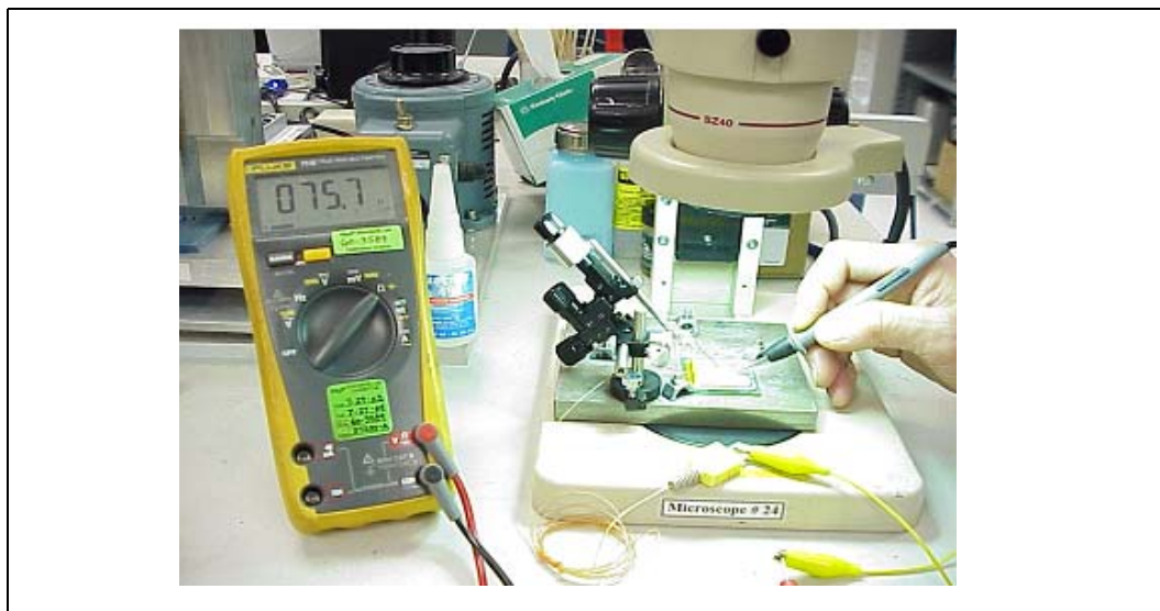
Figure 29. Measuring Resistance between Thermocouple and IHS
