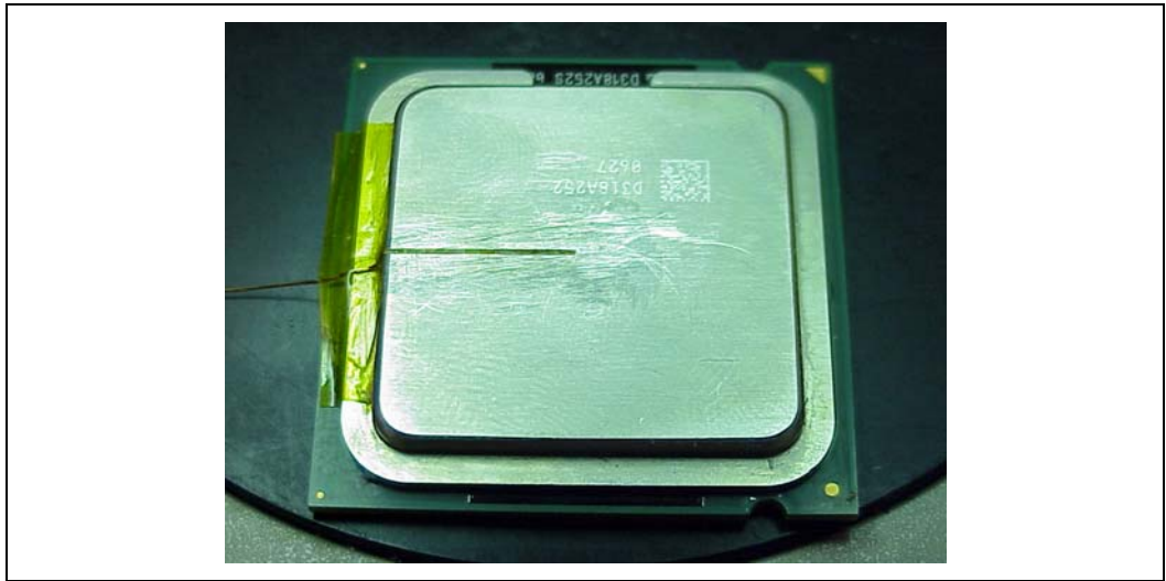
Figure 34. Thermocouple Placed into Groove
