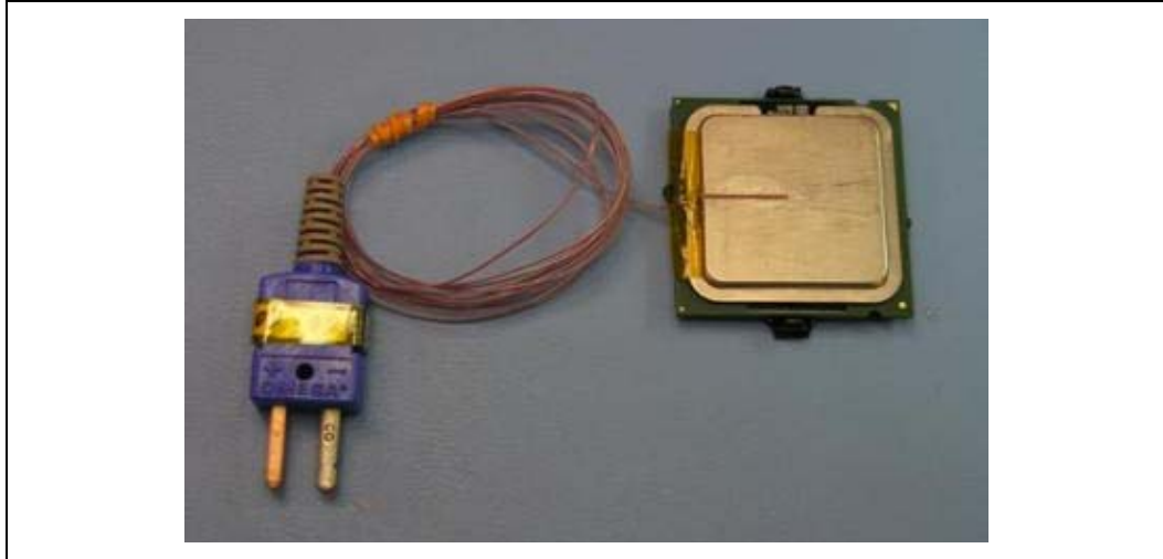
Figure 39. Finished Thermocouple Installation
