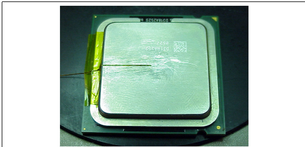
Figure 40. Thermocouple placed into groove
