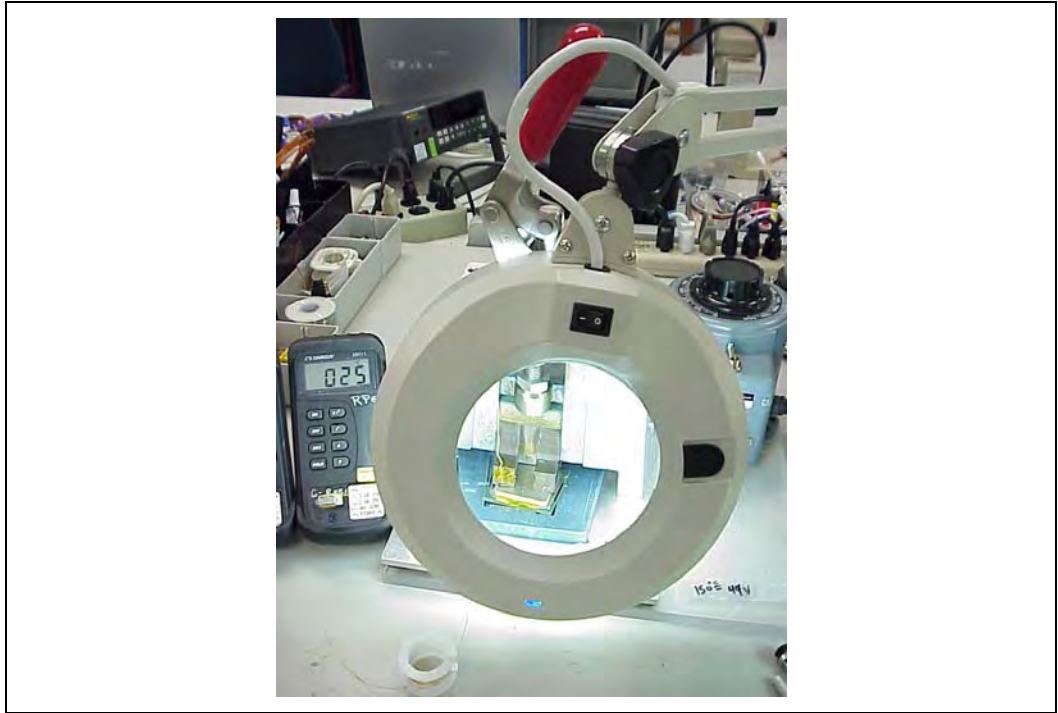
Figure 48. Moving Solder back onto Thermocouple Bead
