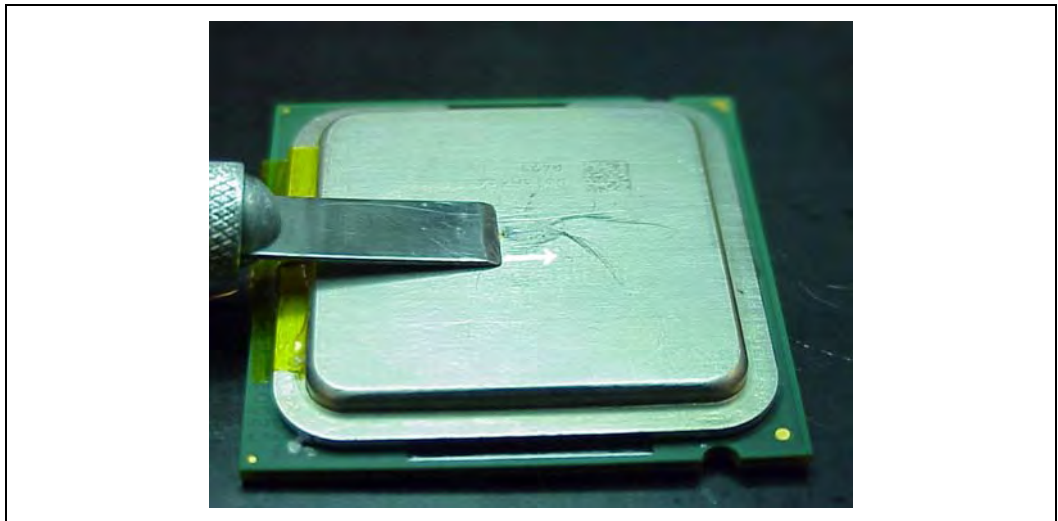
Figure 51. Removing Excess Solder
