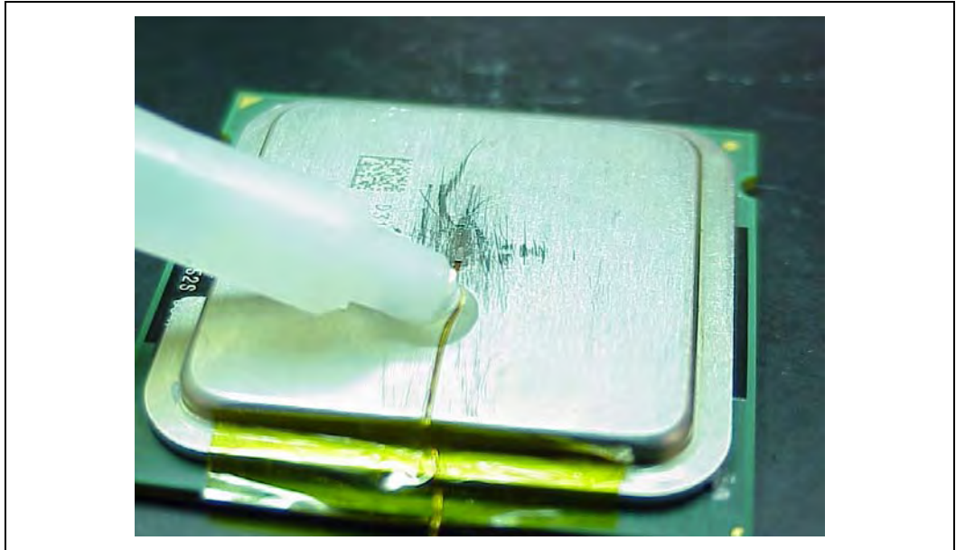
Figure 52. Filling Groove with Adhesive
