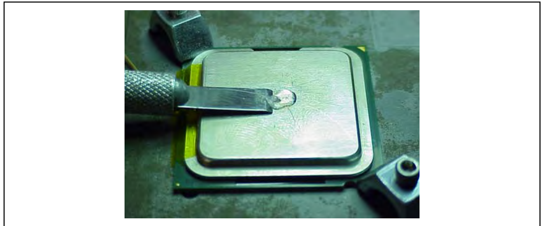
Figure 54. Removing Excess Adhesive from IHS
