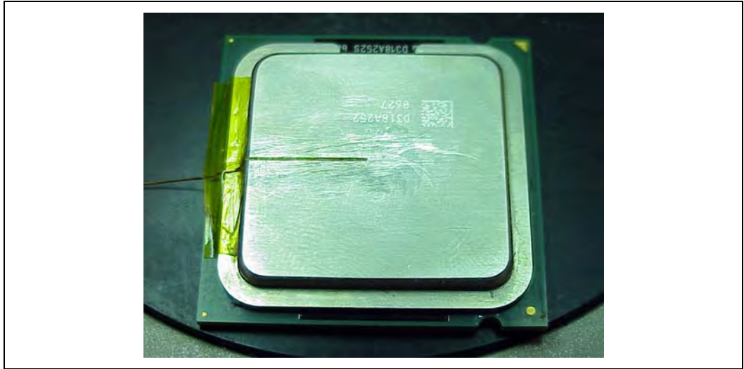
Figure 50. Thermocouple placed into groove
