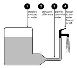
Electrical current in a circuit behaves like water flowing in the water pipes of your house. Getting water to the kitchen sink requires four things: a suitable amount of water, a pipe to carry the water, a pressure difference between the source of the water and the tap, and a tap to turn the flow of water on or off.
