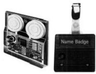
The tab computer, worn as a badge, is equipped with a microprocessor, infrared sensors, transmitters, and batteries (note internal view).
