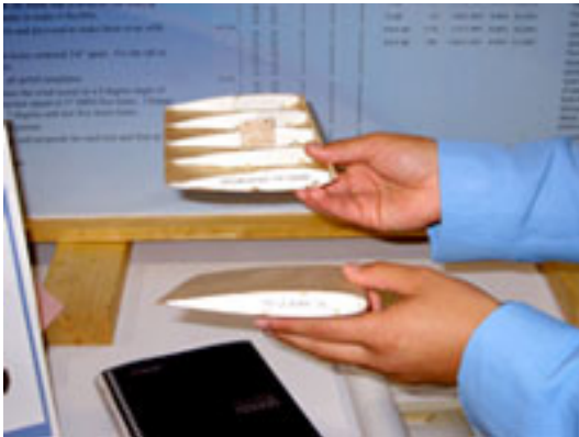
Woodward tested five airfoil sections.
