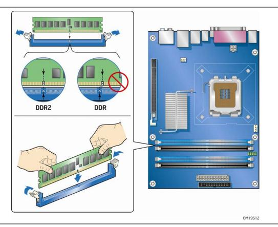
Figure 17. Installing a DIMM
