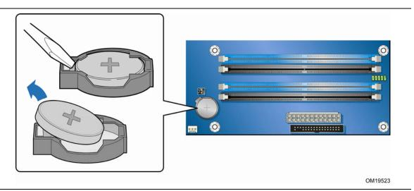
Figure 29. Removing the Battery
