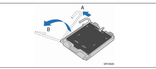
Figure 6. Lift Socket Lever
