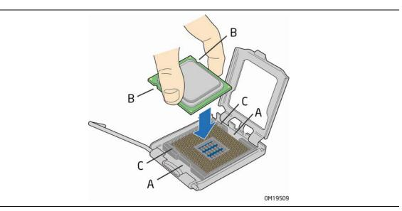
Figure 10. Install the Processor
