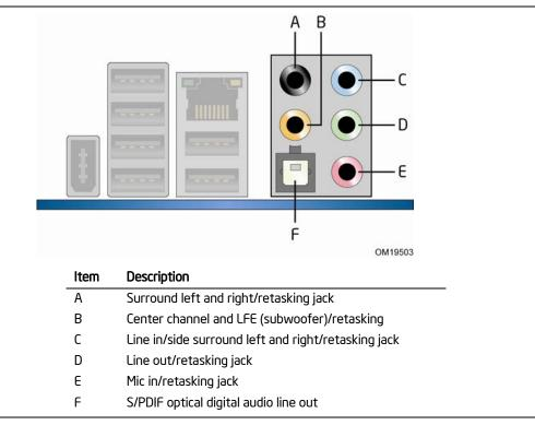
Figure 23. Back Panel Audio Connectors
