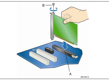
Figure 18. Installing a PCI Express x16 Card
