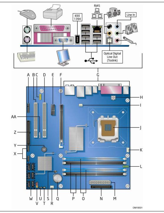
Figure 1. Desktop Board DG965OT Components
