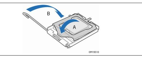
Figure 11. Close the Load Plate
