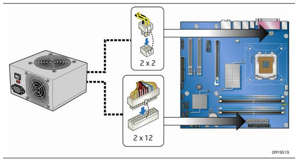
Figure 25. Connecting Power Supply Cables
