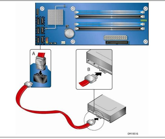
Figure 21. Connecting the Serial ATA Cable
