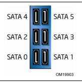
Figure 30. Original SATA Port Mapping for Desktop Board DG9650T
