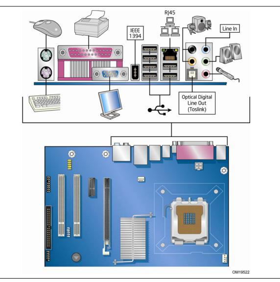
Figure 28. Back Panel Connectors
