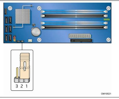
Figure 27. Location of the BIOS Configuration Jumper Block
