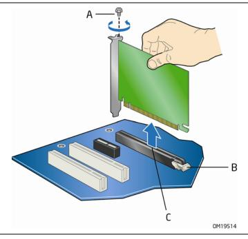
Figure 19. Removing a PCI Express x16 Card
