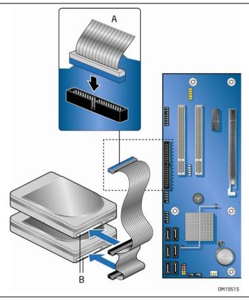
Figure 20. Connecting the IDE Cable
