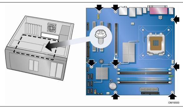
Figure 5 shows the location of the mounting screw holes for Desktop Board DG965OT.
