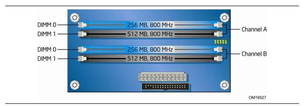
Figure 14. Dual Channel Memory Configuration Example 2
