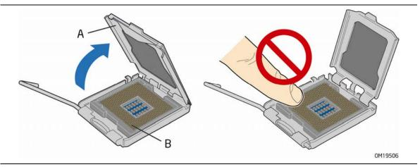
Figure 7. Lift the Load Plate
