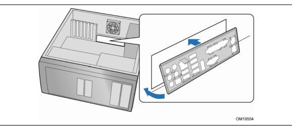
Figure 4. Installing the I/O Shield
