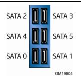
Figure 31. SATA Port Mapping for Desktop Board DG965OT After RAID is Enabled
