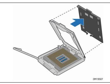
Figure 8. Remove the Protective Socket Cover
