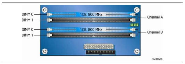
Figure 13. Dual Channel Memory Configuration Example 1
