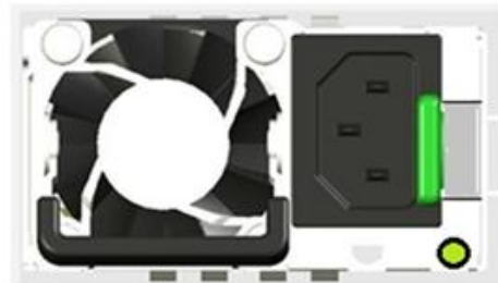
Figure 19. AC Power Supply – Connector View
