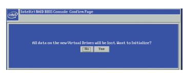
Select **Fast Initialize** to do a preliminary initialization of the drives for loading the operating system. A full initialization will occur in the background.
