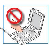
C. Remove the Processor Protective Cover
