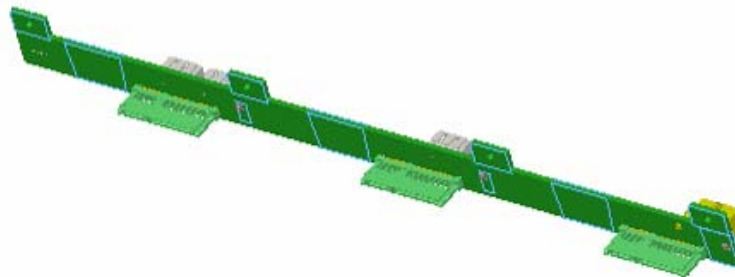
Figure 19. Intel® Server System SR1630HGP Hot-swap Backplane
