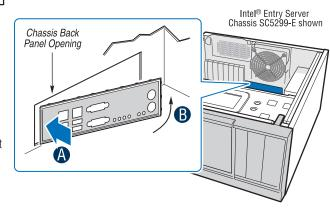
Installing the I/O Shield and Attach I/O Label
