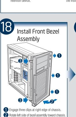
3 Snap two bezel tabs into corresponding
