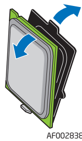
Figure 38. Removing the Processor Protective Cover
