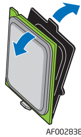
Figure 38. Removing the Processor Protective Cover
