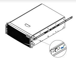
Align inner member key holes to standoffs on chassis, move inner member following the direction in left pictures.
