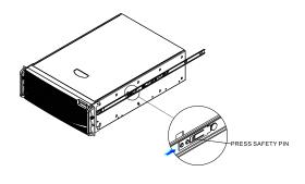
Press safety locking pin to release inner member from chassis.
