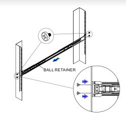
Align brackets to desired vertical position on rack and insert fasteners.
