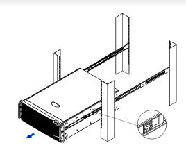
Fully extend the slides until it is in the locked position, pull the release button to release lock and disconnect inner member from slides.
