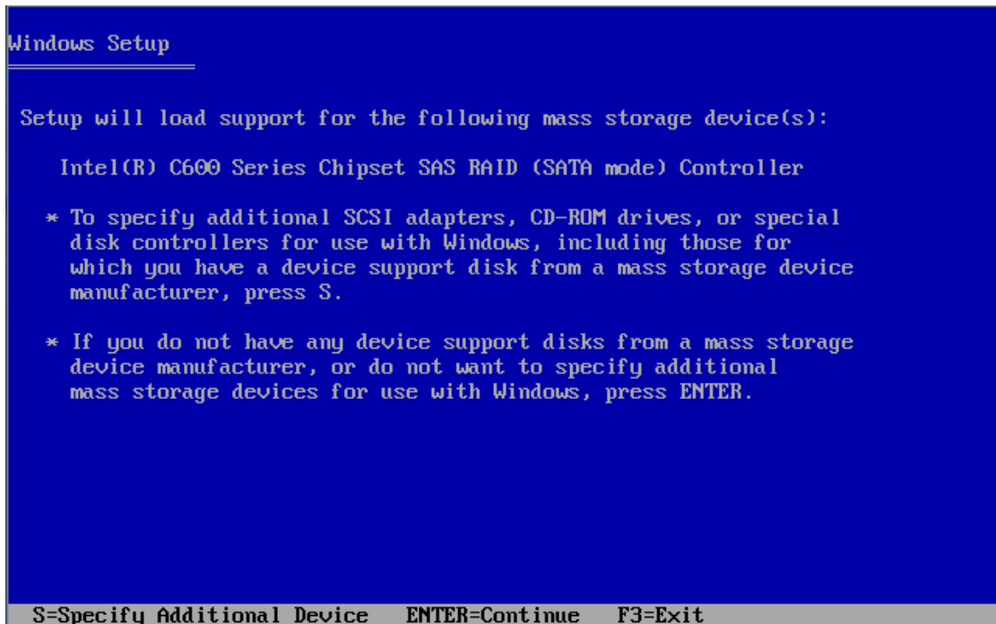
Figure 45. Load Support for Mass Storage Device
