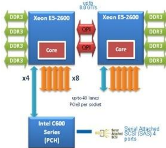
Figure 11. General Functional Block Diagram of Processor I/O Sub-system
