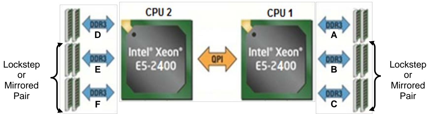
Figure 11. Memory Channel Pairing for RAS Support
