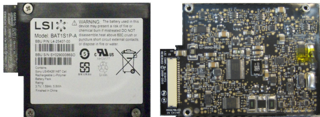
Figure 11. Intel® RAID Smart Battery AXXRSBBU9
