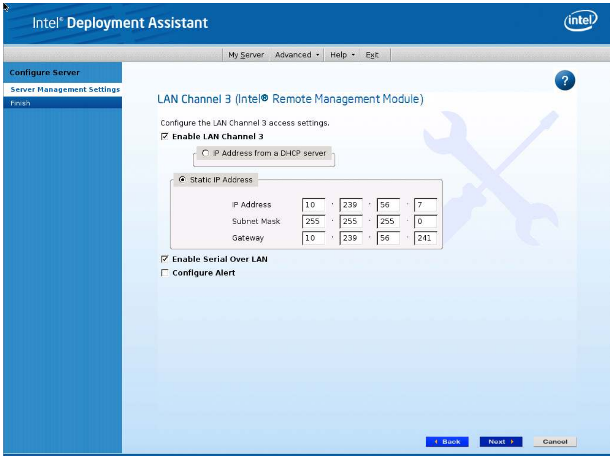
Figure 16: IDA Configure Server: Configure LAN Channel 3 (Intel® RMM4 DMN) Static IP Address window
