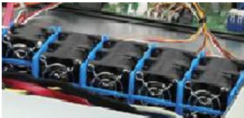
Figure 10. Intel® Server Chassis SC1400UP System Fans 4, 5, 6, 7, 8
