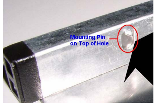
Figure 2: CDROM Tray with correctly oriented pins
