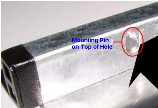
Figure 3: Floppy Tray with misoriented pins
