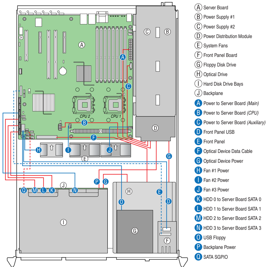
Figure 58. Cable Routing (SR2520SAX/SR2520SAXS and SR2520SAXR/SR2520SAXSR)
