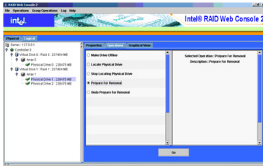
Figure 82. Preparing Drive for Removal
