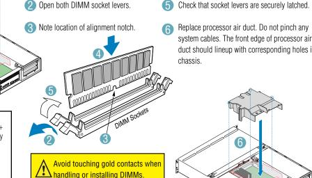
Lift the processor air duct from its
