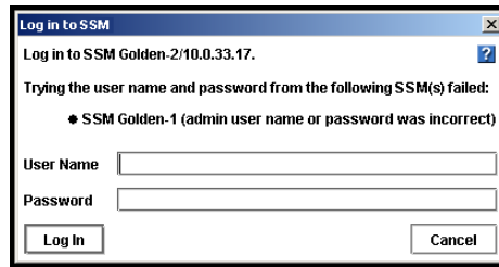
Figure 30. Automatic Log In Fails because SSM User Name and Password are Different
