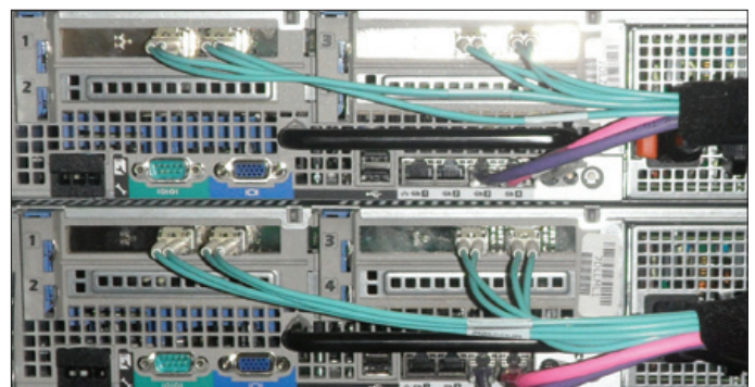
Figure 2. Simplified server connectivity using 10GbE
