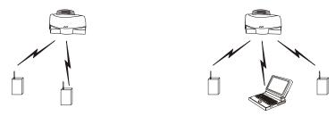
Multiple APs wired together provide a network with better coverage area and performance when using the same Net\_IDs.
