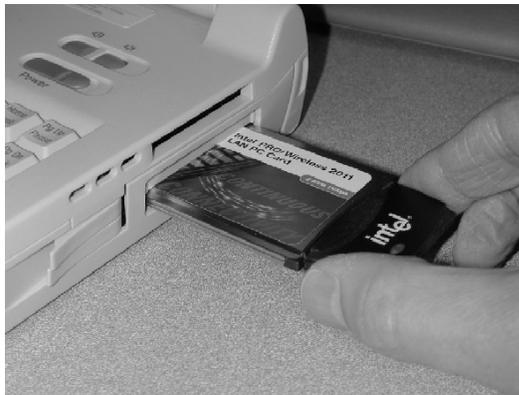
3. When fully inserted the PC Card antenna and LED protrudes as shown below.
