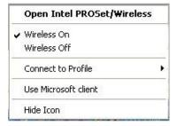
The Intel PROSet/Wireless icon displays in the task tray located in the lower right corner of your Windows desktop. Right-click the status icon to display the menu options. Intel PROSet/Wireless can support multiple adapters. These wireless adapters are displayed in the task tray menu options.
